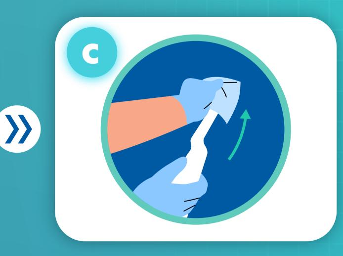
Clean residues/gel from the probe tip/nose.
